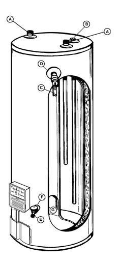
Never use this water heater unless it is completely filled with water. To prevent damage to the tank, the tank must be filled with water. Water must flow from the hot water faucet before turning "ON" gas to the water heater.
